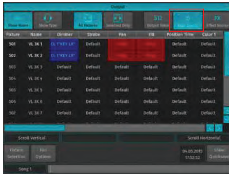
Figure 173: Output Window - Base Source Button
